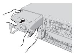
Figure 3. Replacing the Power Supply
